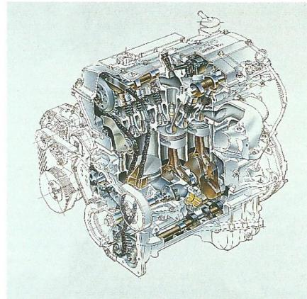
The 2.3i has a specially-designed twin balancer shaft assembly, which cuts mechanical noise intrusion to the interior of the vehicle.
