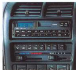
2007 or 2006R RDS Audio Systems with Keycode security and vehicle registration memory.
