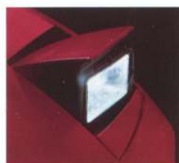
Retractable headlights conveniently retract when not in use, protecting the glass from dirt and damage.
