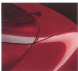
Tailgate wiper with electric wash essential for allowing greater rear visibility.
