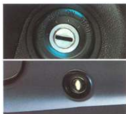
Illuminated ignition and locks designed for locating locks in failing light or darkness.
