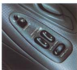
Control panel for power windows in door ensures convenient ease of operation.
