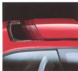
Electrically-operated sliding sunroof to take advantage of sunshine and fresh air.
