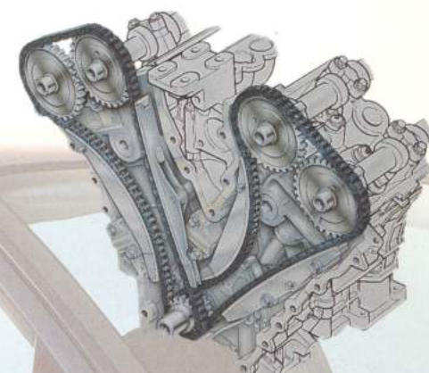
The double overhead camshafts for each cylinder head are driven off the crankshaft by a silent chain drive with patented automatic hydraulic tensioners to keep valve timing accurate and reduce operating noise.
