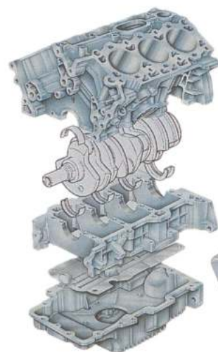
The crankshaft is split on the bearing centre-line with four forged-steel main bearing caps cast in a separate aluminium die-cast bridge (known as a girdle).
