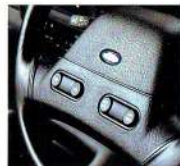
Cruise control buttons conveniently located on steering wheel boss.
