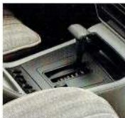
Four speed electronically controlled automatic transmission with 'power' and 'economy' modes.
