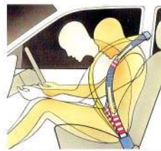
Belt-locator device instantly minimises payout of seat belt webbing.
