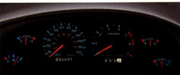
Mustang comes equipped with analogue gauges: engine temperature, battery charge, fuel level and oil pressure. Plus a tachometer to read the pulse of the standard 3.8-litre V-6.
