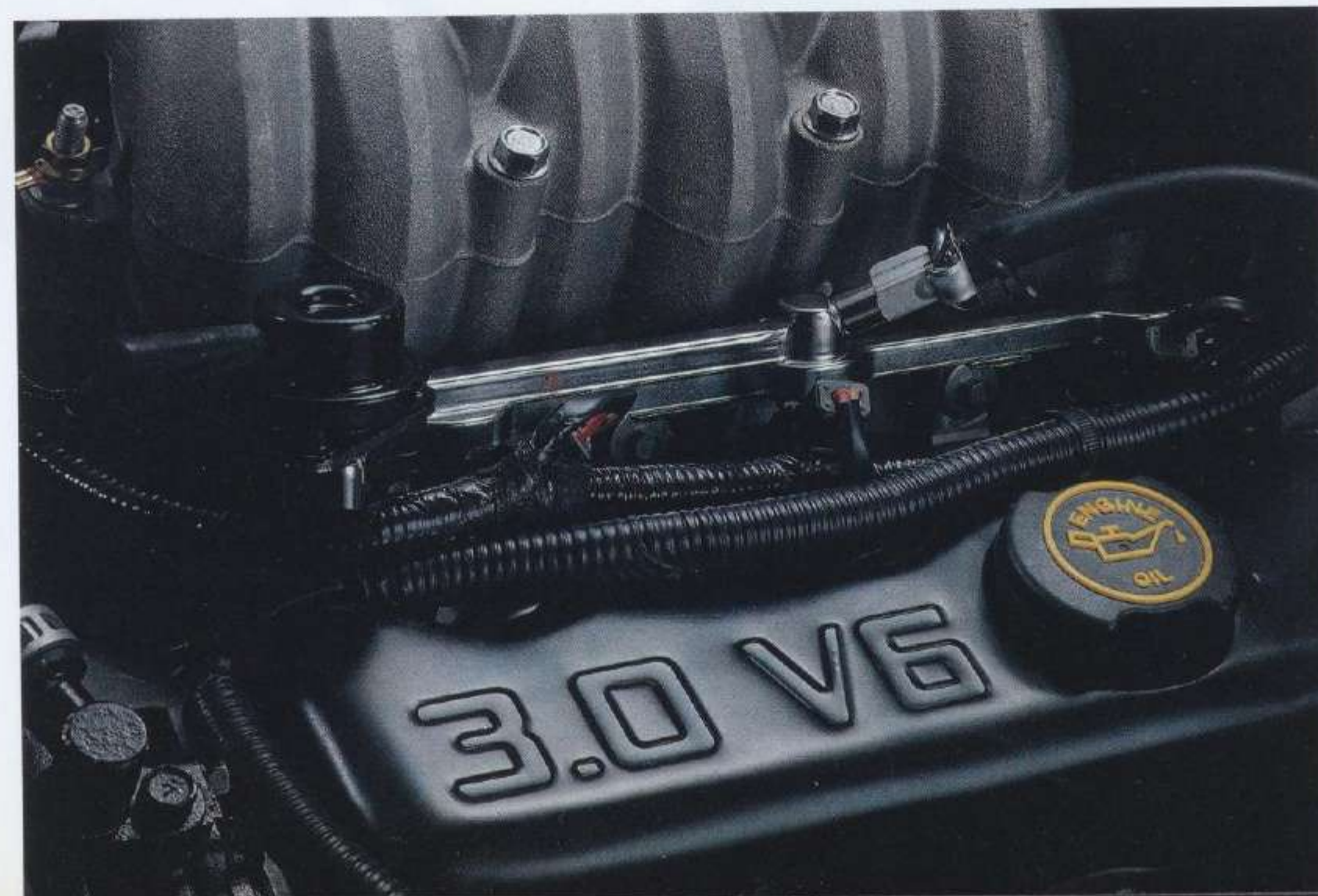
The 3.0L V-6, standard in Probe LX, features 12-in. tuned air intake runners and a multi-port electronic fuel-injection system controlled by the EEC-IV computer.
