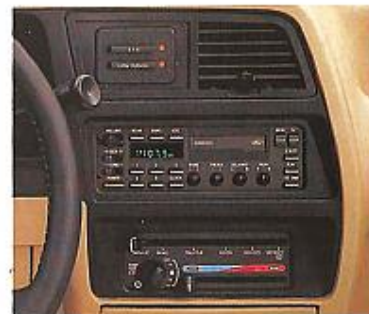
In a pod to the right of the instrument cluster are, from top to bottom: (1) the push-button control module for the Touch Drive electric shift transfer case, standard in Explorer 4x4 models; (2) the stereo system; and (3) the heating/cooling/defroster system controls.
