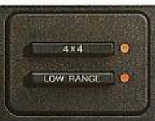
Push-button controls for the standard Touch Drive electric shift transfer case (in the 4x4 model) are on the instrument panel — a more convenient arrangement than the floor-mounted shift found in other 4x4 compact utility vehicles.
