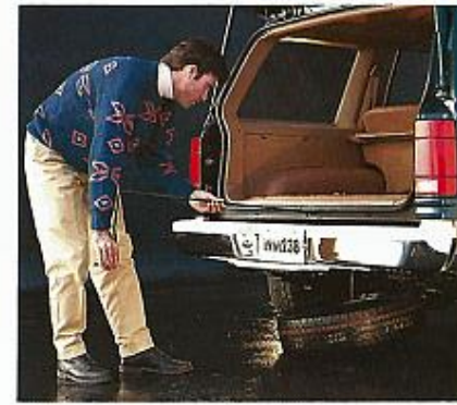
The standard full-size spare tire is mounted to the frame between the rear frame rails. This design allows for increased cargo space. The tire lowers easily with a crank mechanism.
