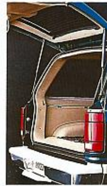
You can access Explorer's spacious cargo compartment from the rear by raising the entire steel liftgate or just the window. Both open with the assist of pneumatic struts. A pull-down handle is included.
