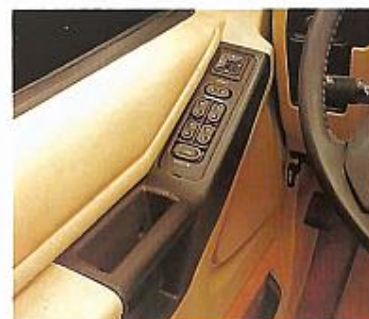
Features of the optional power equipment group (power door locks, windows, and electric remote-control mirrors) are located on a special ergonomic door-mounted panel. Tactile controls, easily identified by touch alone, are designed with a "bump" at one end ("on") and a "dimple" at the other end ("off").
