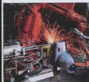
Automated welding and brazing provide consistent precision and accuracy for body construction.
