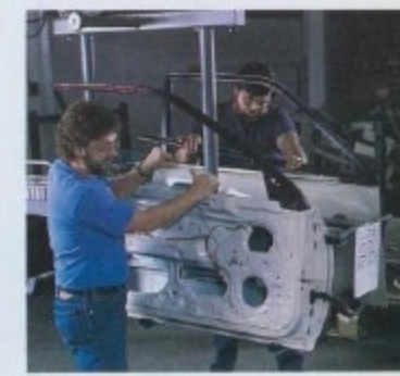
Doors are precision-fitted, removed from the body and re-hung later. This prevents damage and makes the interior more accessible to assemblers.
