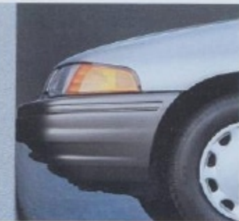
Escort's wraparound bumpers are built to withstand impacts of 5 mph, exceeding Federal Government requirements.
