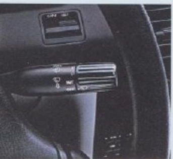
The windshield wiper system has been redesigned to include a fixed interval feature that's handy in light rain and drizzle.
