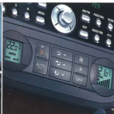
Dual Electronic Automatic Temperature Control (DEATC) provides easy-to-use separate driver and passenger temperature controls to keep all occupants comfortable. (Optional on Zetec and Ghia.)
