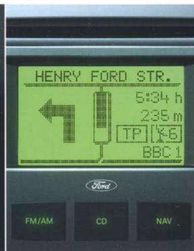
Blaupunkt radio navigation system provides visual and spoken directions to your selected destination and features a monochrome display.
