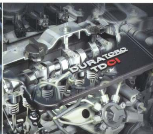
TDCi Powerful and refined, the new 115 PS 1.8-litre Duratorq TDCi diesel engine.
