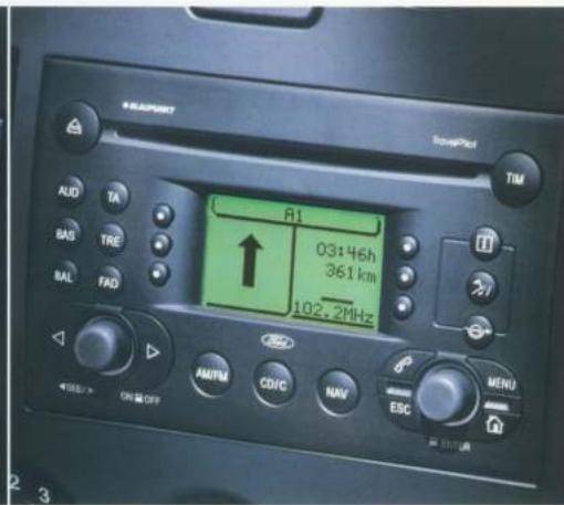
Satellite navigation Combining a radio, CD player and guidance system, the optional Travel Pilot navigation system will suggest the best route to your destination and guide you with a friendly voice and visual directions. Available on selected models as an option at extra cost.
