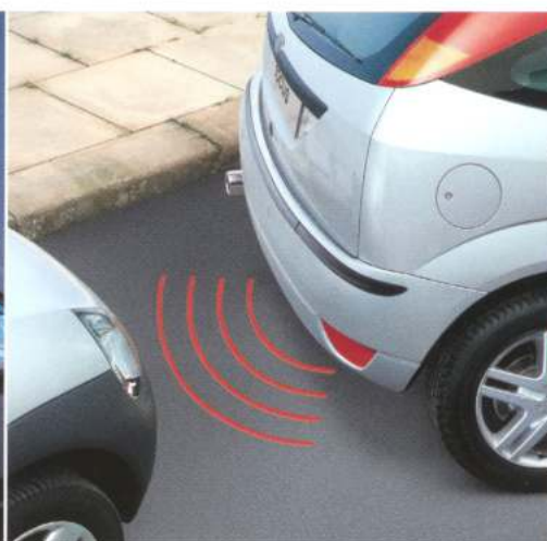
Park Assist sensors located in the rear bumper help the driver to safely judge parking distances by means of an audible warning.
