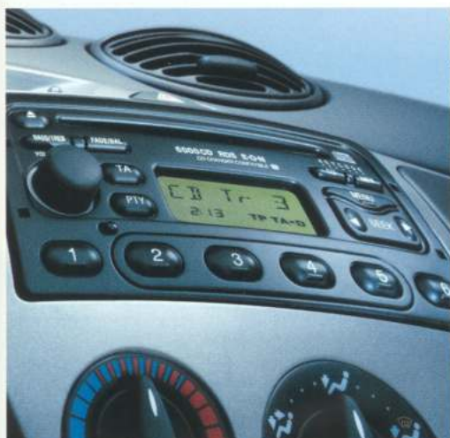
Model 6000N RDS EON with remote column-mounted controls, removable control panel, 'Keycode' anti-theft coding, 4 speakers.
