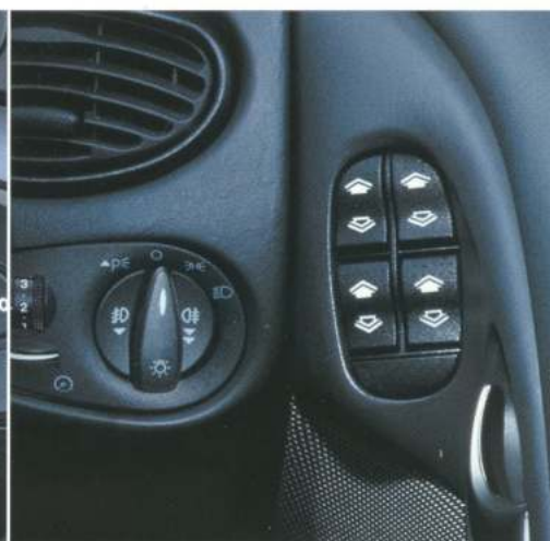
Electrically-operated front and rear windows feature 'bounce-back' sensors for safety.
