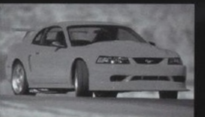
2000 SVT Mustang Cobra R 385 horsepower 5.4-liter dohc V8 Tremec six-speed manual transmission Lightweight street-legal racing model Production: 300 units
