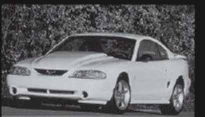
1995 SVT Mustang Cobra R 300 horsepower 5.8-liter ohv V8 Tremec five-speed manual transmission Lightweight street-legal racing model Production: 250 units
