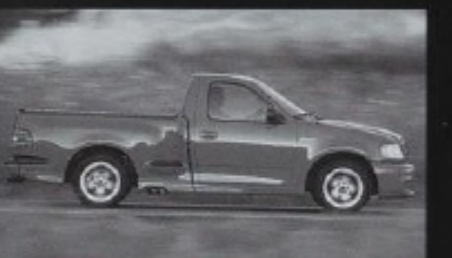
1999-2001 SVT F-150 Lightning 360 hp ('99-'00) 380 hp ('01) supercharged 5.4-liter Triton™ V8 Four-wheel disc brakes introduced 5,000-pound tow rating Production: 15,346 units (est.)
