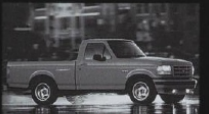
1993-1995 SVT F-150 Lightning 240 horsepower 5.8-liter ohv V8 E40D four-speed automatic transmission Tow rating: 5,000 lbs.; payload: 745 lbs. Production: 11,563 units
