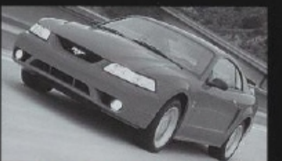
1999 SVT Mustang Cobra 320 horsepower 4.6-liter dohc V8 Independent rear suspension introduced Traction control introduced Production: 8,095 units
