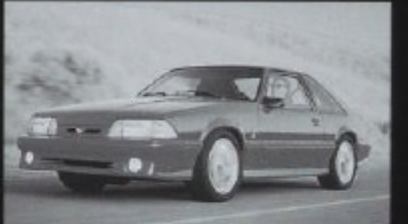
1993 SVT Mustang Cobra 235 horsepower 5.0-liter ohv V8 T5 five-speed manual transmission Four-wheel disc brakes Production: 4,993 units
