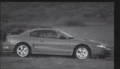
1996-1998 SVT Mustang Cobra 305 horsepower 4.6-liter dohc V8 T45 five-speed manual transmission 13-in. front discs, PBR calipers; 11.65-in. rears Production: 28,709 units
