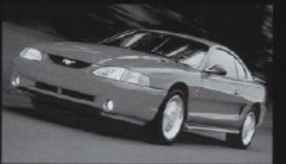
1994-1995 SVT Mustang Cobra 240 horsepower 5.0-liter ohv V8 T5 five-speed manual transmission 13-in. front discs, PBR calipers; 11.65-in. rears Production: 11,017 units
