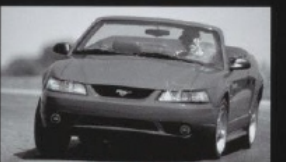
2001 SVT Mustang Cobra 4.6-liter dohc V8, 320 hp @ 6,000 rpm 317 lb.-ft. torque @ 4,750 rpm. Traction control standard Production: 7,251 units (est.)
