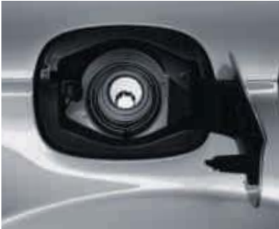
Capless refuelling with Ford Easy-Fuel No dirty fuel caps to touch. Ford Easy-Fuel with its unique safeguard ensures nobody accidentally fills up with the wrong fuel. (Standard)
