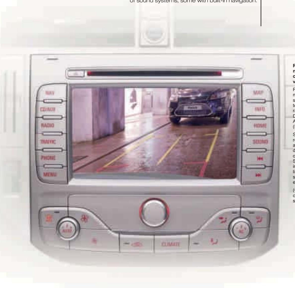
Radio/CD/premium SD-navigation system with 7" colour touchscreen and rear-view camera
