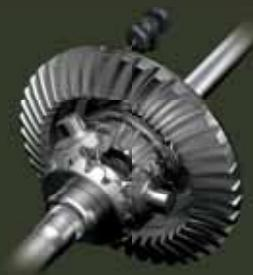
■ An available **ELECTRONIC-LOCKING REAR DIFFERENTIAL** uses a true mechanical dog-clutch mechanism to lock both rear axle shafts together so they turn at the same speed for maximum traction.
