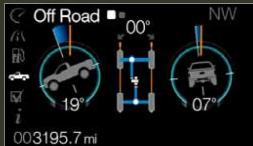
■ Monitor pitch angle, bank angle and wheel direction with the **CLASS-EXCLUSIVE OFF-ROAD DISPLAY** in the available LCD productivity screen.
