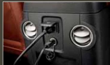
**110-VOLT POWER INVERTER** is conveniently located on the back of the available center console.
