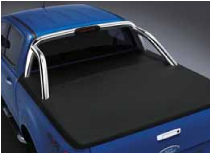
EGR soft tonneau cover. Helps protect equipment and valuables from rain and dust.
