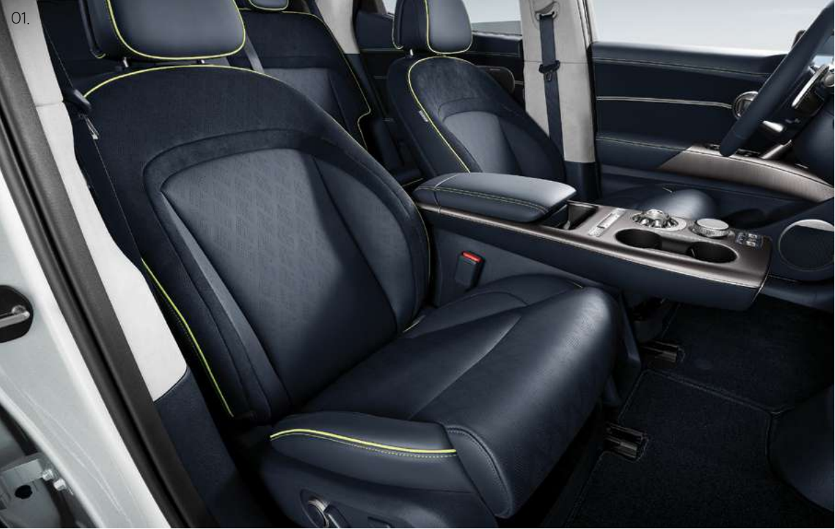
01. Front Relaxation Comfort Seats _ The driver and passenger seats both utilize the relaxation comfort seat technology to lower fatigue and increase comfort by positioning passengers in an optimal, zero-gravity position that relieves pressure on the body to create a truly relaxing ride.
