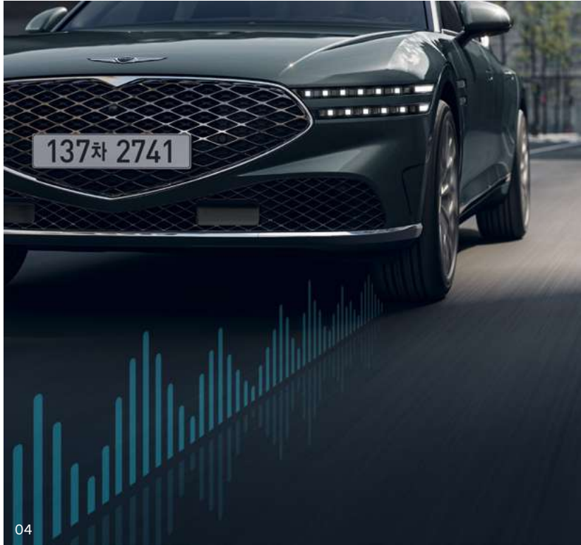
04. Active Noise Control-Road (ANC-R) _ This system cancels road noise that enters the cabin by sending inverted sound waves, reducing road noise and increasing tranquility in the cabin.
