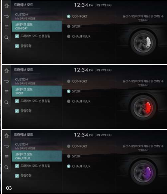
03. Brake mode _ Drivers can choose between three brake modes: Comfort mode aims for comfortable and stable braking; Sport mode seeks to deliver quick responsiveness and sporty braking; and the new Chauffeur mode pursues optimal comfort for the rear seat passengers.
