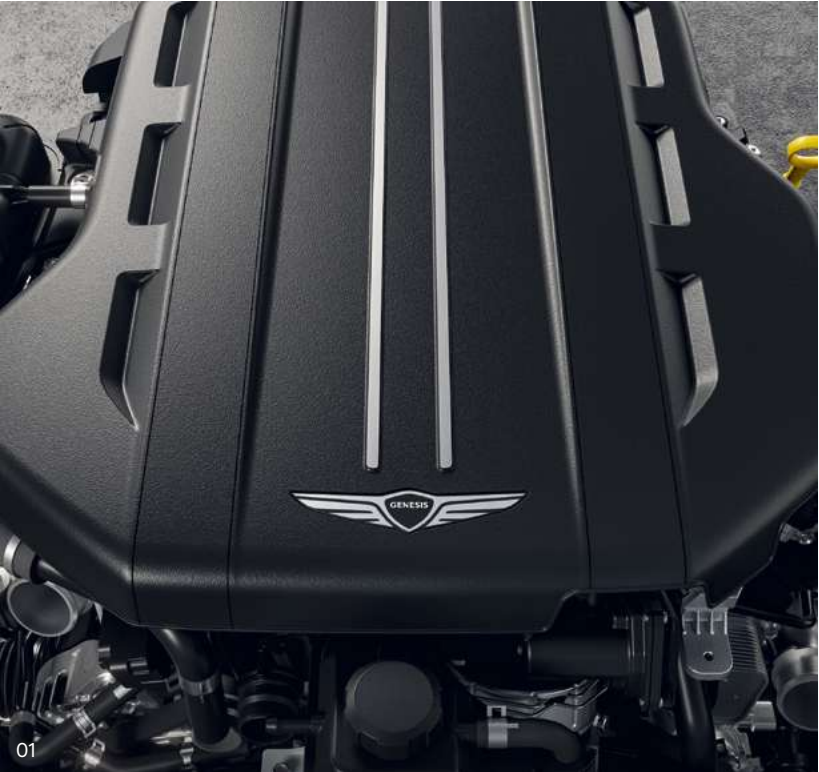
01. 3.5 turbo gasoline engine _ Dynamic driving is achieved with solid power and torque, while the air-to-water intercooler improves fuel economy and responsiveness.
