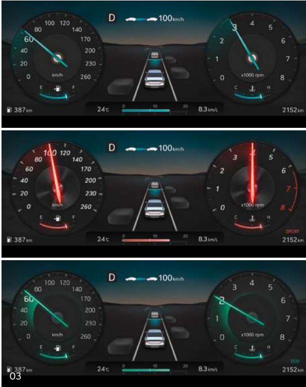
03. Drive mode control system _ Drivers can switch between Comfort, Eco, Sport, or Custom driving modes according to preferences or driving conditions. From the smooth ride of the comfort mode to the powerful acceleration of the sports mode and to the fuel efficient eco mode, Genesis G90 is ready to deliver optimal driving for any situation.
