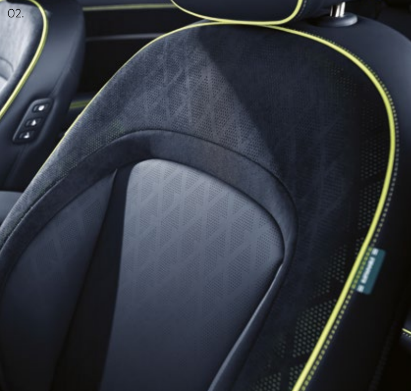
02. ERGO Motion Driver Seat _ The driver’s seat features ERGO Motion seat technology, linked with the drive mode or speed set by the driver, that uses air-cells within the seat to enhance support on the sides and seat cushion for optimal comfort. Stretching mode is also available and adjusts the air-cells one by one, thus reducing driving fatigue.
