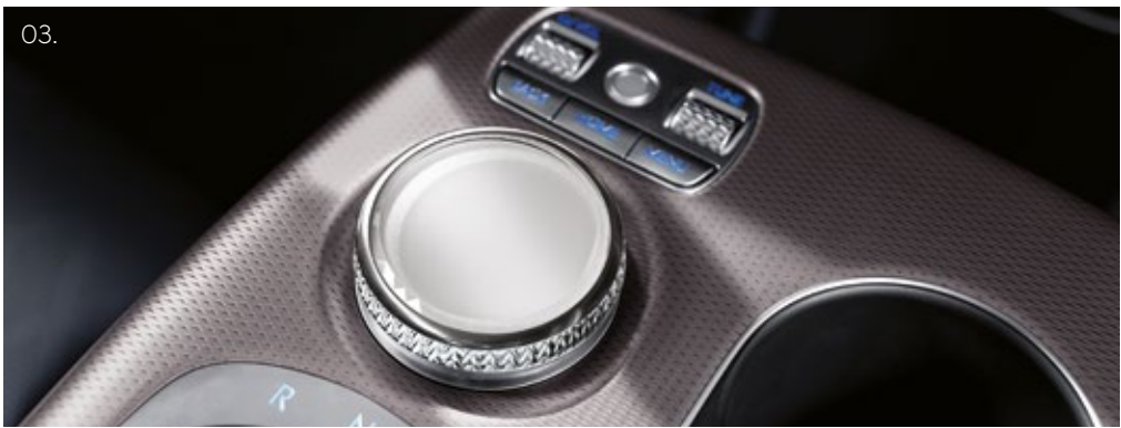
02. 03. Diffuser (Front Passenger Door Handle) _ Inserted into the front passenger door’s handle, the membrane-type diffuser is a subtle detail that contributes to the classy atmosphere and keeps the interior feeling fresh. GENESIS Touch Controller _ Located in the center console, the controller allows users to utilize the various infotainment systems easily at the touch of a finger. Its handwriting recognition system allows users to enter a destination or search for a phone number without a keyboard by simply writing it.
