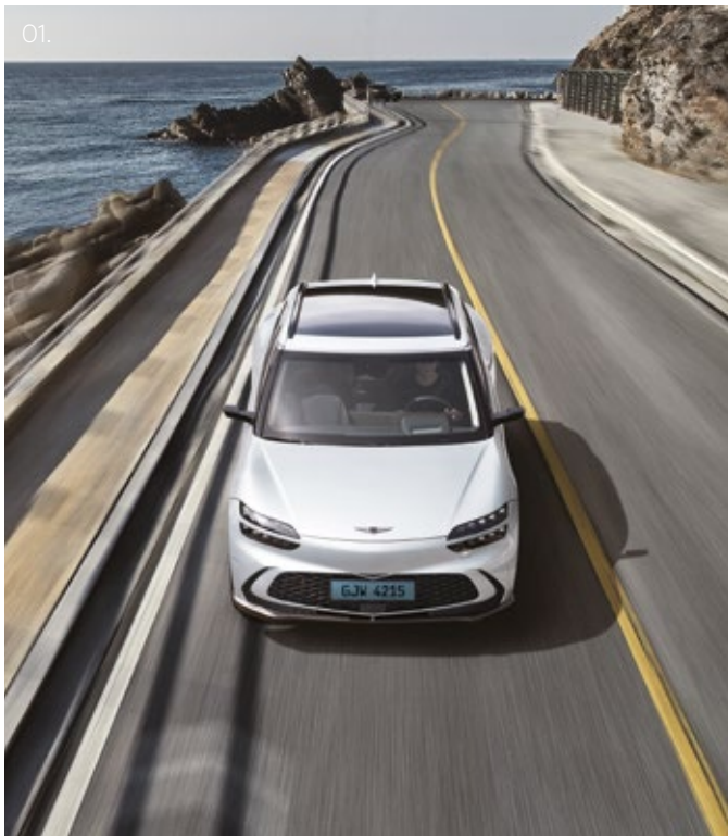
01. Lane Following Assist (LFA) _ Assists with steering to keep the vehicle centered in its current lane.
