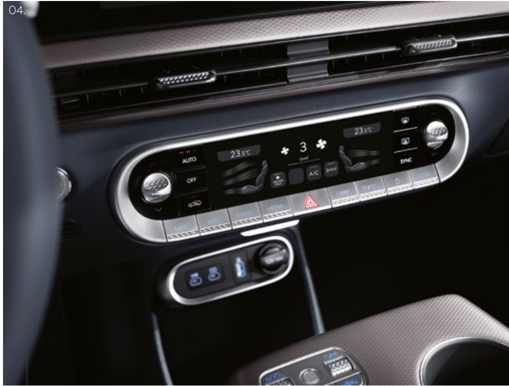
04. Fully Independent Automatic Air Conditioning (Dual Driver/Passenger Climate Control, Auto De-fog, Outside Airflow Prevention) _ Controls the temperature and airflow to maintain a comfortable and enjoyable interior atmosphere in all four seasons.
