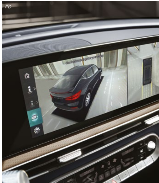
02. Surround View Monitor (SVM) _ Video images of the area around the vehicle can be viewed to assist with safe parking.
