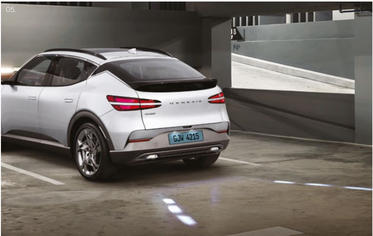
05. Reverse Guide Lamps _ When the vehicle is in reverse, the guide lights illuminate the road behind the vehicle so that people and other vehicles can easily notice the driver's intention to back up and to minimize the risk of accidents.
