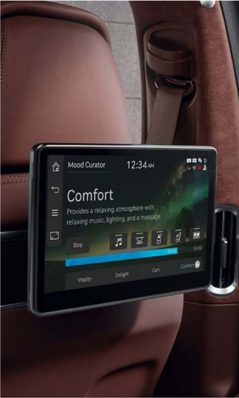
Mood curator _ Creates four different moods (vitality, delight, care, comfort) via integrated control of the vehicle's audio system, fragrance, ambient lights, curtains, and massage function.
