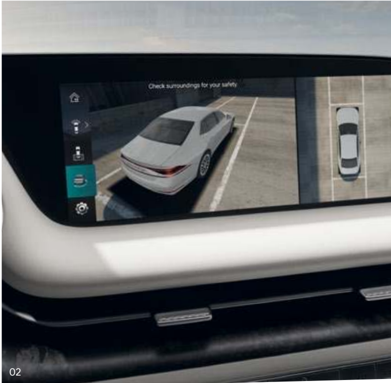
02. Surround View Monitor (SVM) system _ Video images of the area surrounding the vehicle can be viewed to assist in safe parking.
