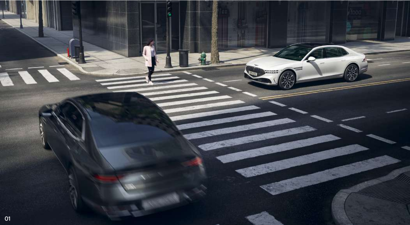
01. Forward Collision-Avoidance Assist 2 (FCA) system _ When a collision risk with a vehicle/pedestrian/bicycle ahead is detected, this system warns the driver and, if necessary, helps to control the brake to avoid a collision. When there is a collision risk with vehicles approaching from left/right sides of an intersection, it automatically assists in braking. It also assists in steering if there is a collision risk when changing lanes.
