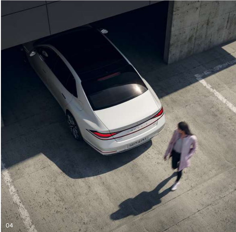
04. Parking Collision-Avoidance Assist (PCA) system (front/side/rear) _ It sounds a warning if there is a collision risk with nearby pedestrians or objects while parking or exiting a parking spot. If the risk continues after the warning, it automatically assists in braking.
