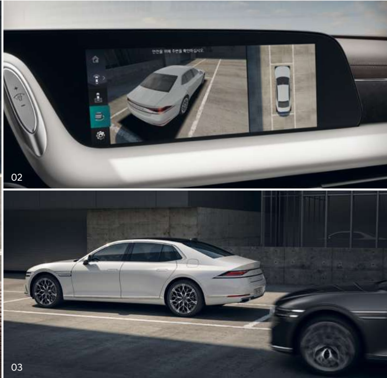
02. Surround View Monitor (SVM) system _ Video images of the area surrounding the vehicle can be viewed to assist in safe parking. 03. Safe Exit Assist (SEA) system _ When passengers are about to exit a parked vehicle, SEA detects vehicles approaching from the side rear and sends a warning. It also keeps the Electronic Child Safety Lock activated to prevent the doors from opening. In addition, if the risk of a rear side collision is detected, the door is prevented from opening even if the open button is pressed.
