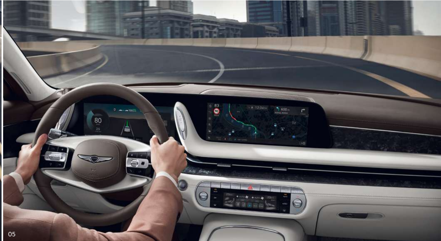
05. Navigation-based Smart Cruise Control (NSCC) system _ This system automatically slows down the vehicle upon entering a limited speed zone area or a curved section, returning to its previous set speed afterwards. It also reduces the speed when entering/exiting a highway, assisting in safe driving. Highway Driving Assist 2 (HDA) system (includes lane changing assist) _ While on the highway, this helps the vehicle maintain a safe distance from the vehicle in front and also to stay centered in its lane at a set speed even in curved sections. It also assists in lane changes.
