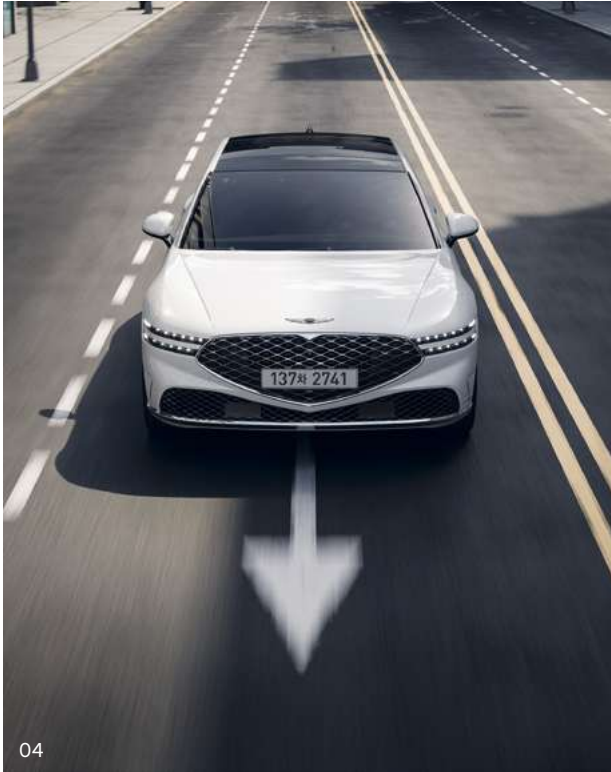
04. Lane Keeping Assist (LKA) system _ It warns the driver when the vehicle departs from its lane without the use of turn signals and automatically helps steering to keep the vehicle in its lane. Lane Following Assist (LFA) system _ This helps assist steering to keep the vehicle centered in its current lane.
