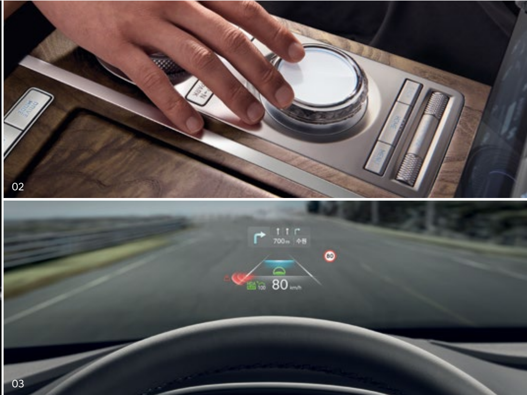
02. 03. GENESIS touch controller _ Located on the center console, this allows users to control the various infotainment systems easily without having to repeatedly touch any buttons or screens. Its handwriting recognition system helps users set a destination or enter a phone number simply by using handwritings instead of typing into a keyboard. Head-Up Display _ Shows driving speed and GPS information, as well as key driver assist information and crossroads. The high-resolution, 12" wide display boasts clear visibility during daytime or nighttime.
