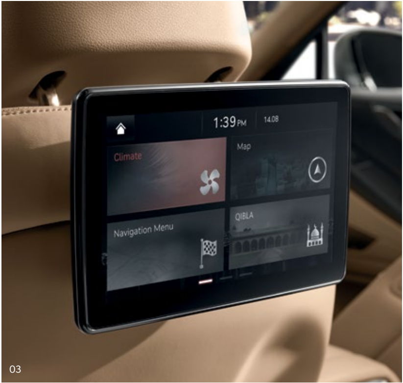
03. Rear seat dual monitors _ The dual rear seat displays consist of large 9.2" monitors that have a wide viewing angle. The monitors allow right and left rear seat passengers to use separate video and audio inputs. Touchscreen features make the monitors easy to use, while the monitors can be tilted to compensate for front-seat adjustments.
