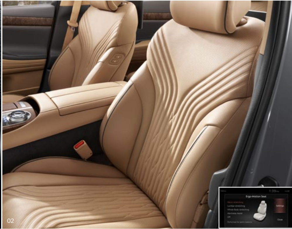
02. ERGO motion driver and passenger seats _ The driver seat and the passenger seat is equipped with ERGO motion seats featuring seven air cells that can be controlled individually to provide optimal seating. Linked to a drive mode or a speed set by the driver, this ergonomic feature can control lateral support. It also offers a stretching mode to reduce fatigue.
