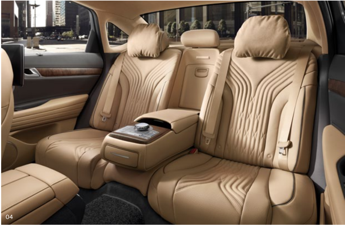
04. Power and ventilated/heated rear seats _ The rear seats can slide forwards or backwards for adjustment while the seats' heating and ventilation system is linked to the vehicle's speed, which automatically controls the blower speed to provide passengers with more meticulous care. The driver can also easily control heating/ventilation of all seats via the main climate control panel.
