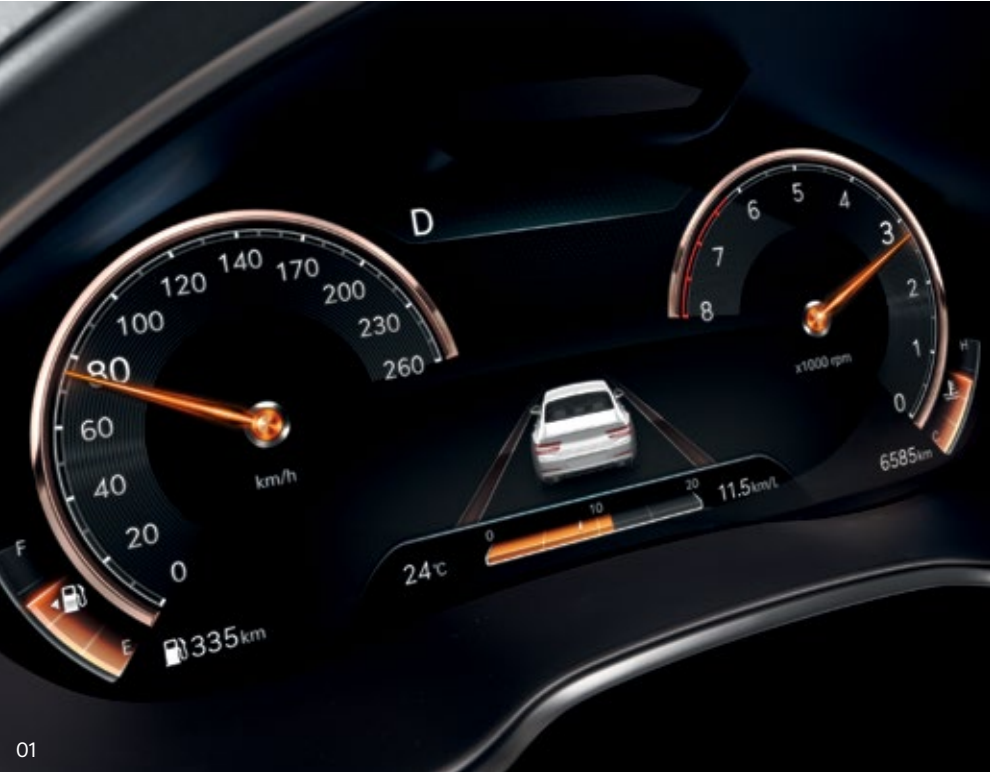
01. 12.3" 3D cluster _ The wide, high-resolution 12.3" 3D cluster provides various view modes and differentiated drive mode illumination. The cluster's embedded camera tracks the driver's eye movements to provide 3D information at any angle, maximizing visibility.
