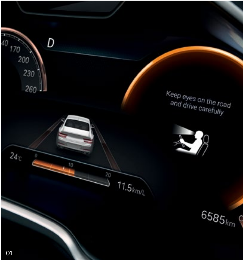
01. Forward Attention Warning (FAW) _ This system alerts the driver if inattentive driving patterns are detected.
