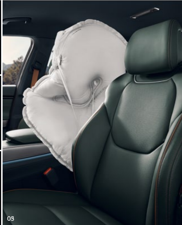
05. 8-airbag system _ In case of a side impact, a center side airbag between the front occupants mitigates impact with each other or with interior materials. Advanced airbags in the driver and front passenger seats deploy after sensing the severity of the impact and the presence of other passengers, while driver's knee airbags, front side-curtain, and rollover-activated side-curtain airbags protect passengers against collisions.
