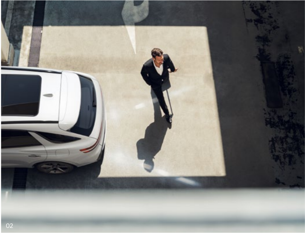
02. Reverse Parking Collision-Avoidance Assist (PCA) system _ This alerts the driver if a collision risk is detected while reversing. If the risk increases even after the warning, it automatically brings the vehicle to a stop.
