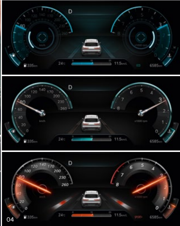
04. Drive mode control system _ Drivers can choose from Eco, Comfort, Custom, Sport, and Sport+ drive modes, depending on driver preferences and road conditions. Each mode delivers optimal driving performance befitting an urban premium SUV: Eco for fuel efficiency, Comfort for smooth driving, Sport and Sport+ for performance and responsiveness. ※ Sport+ mode available with the Sport trims
