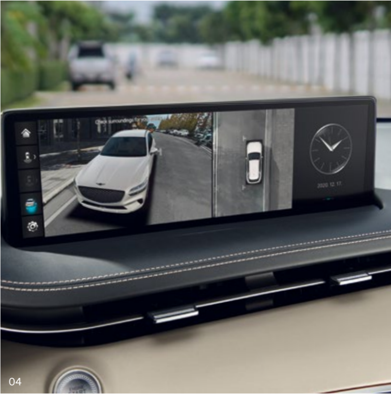
04. Surround View Monitor (SVM) system _ Cameras mounted on the vehicle show diverse images of the vehicle's surroundings, including 3D, 360-degree images from any point of your vehicle, to assist with parking.
