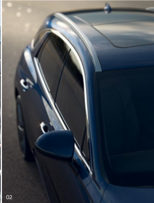
02. Double-jointed soundproof glass _ Acoustically-laminated glass is applied to the front windshield and all doors of the GENESIS GV70 along with improved, triple-layer door sealings to minimize wind noise and maximize noise insulation. Class-leading interior tranquility lets passengers focus on high-quality audio, or on conversations, even at high driving speeds.
