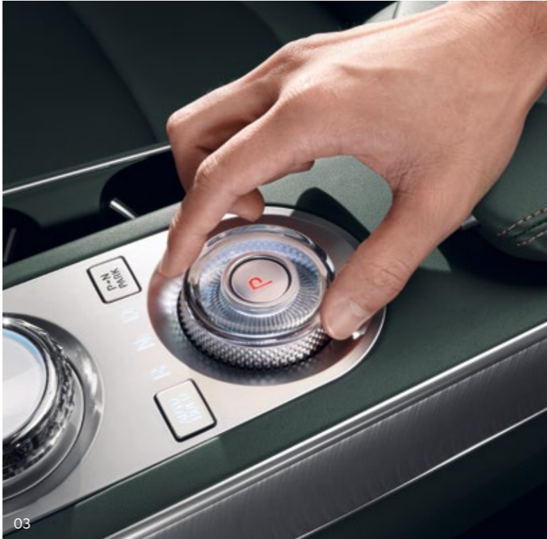
03. 8-speed automatic transmission & Shift-by-Wire (SBW) _ Delivering excellent responsiveness, GV70's 8-speed transmission provides great acceleration from a standstill and optimal fuel economy. The new dial-type Shift By Wire (SBW), made with real tempered glass, offers a firm touch with its flat springs and rolling structure. Ambient lights reveal the beauty of the dial's delicate woven patterns.
