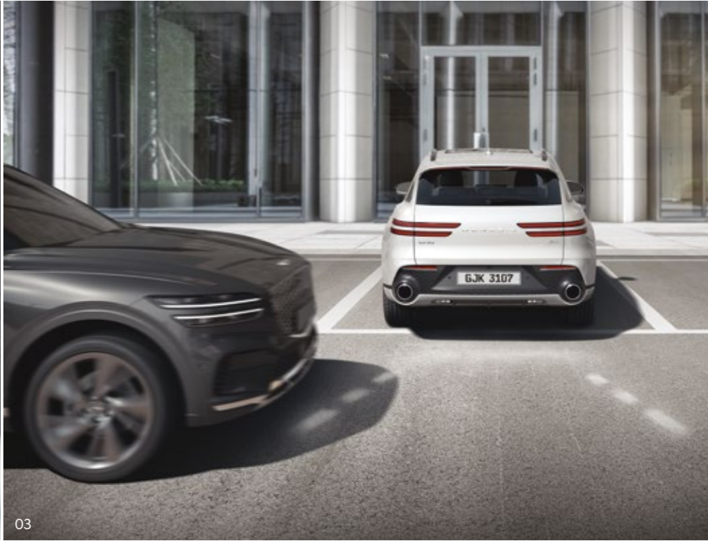
03. Rear Cross-Traffic Collision-Avoidance Assist (RCCA) system _ When in reverse, this alerts the driver if there are vehicles approaching from either side and assists in braking if there is a collision risk.
