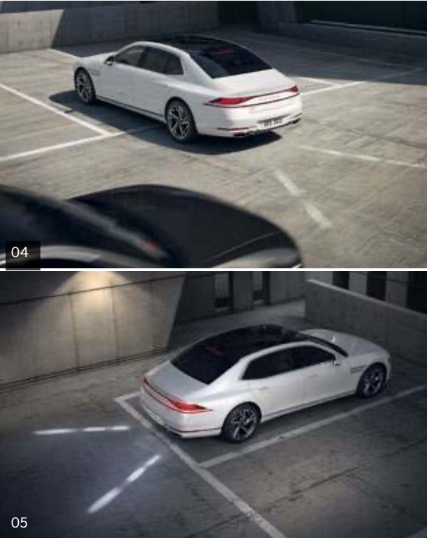
04. 05. Rear Cross-Traffic Collision-Avoidance Assist (RCCA) system _ This alerts the driver if there are vehicles approaching from either side while in reverse. If the risk increases it automatically helps braking. Reverse guiding lamps _ When in reverse, these lights are angled to illuminate the ground behind the vehicle, notifying nearby pedestrians and other vehicles that the vehicle is reversing.
