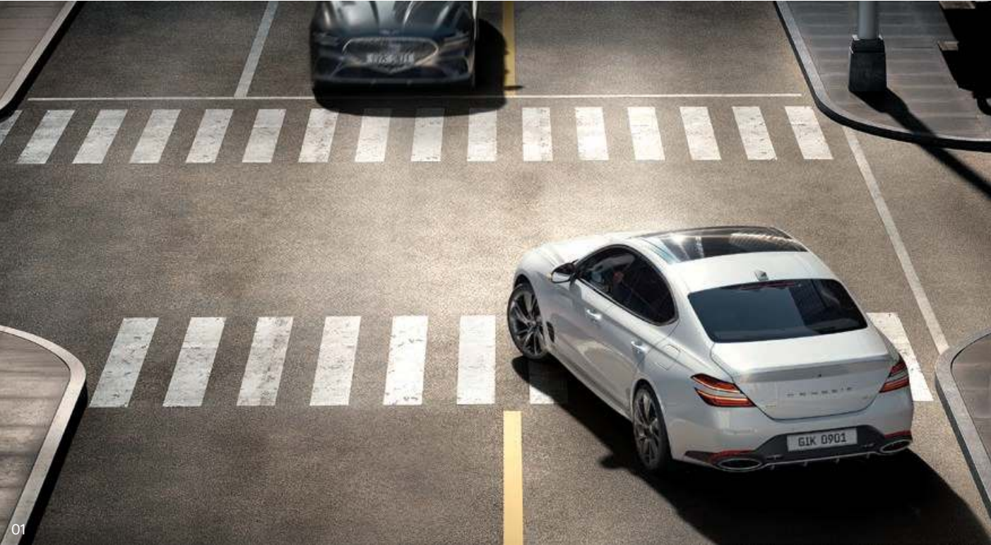
01. Forward Collision-Avoidance Assist (FCA) system (junction turning) _ This system helps to automatically bring the vehicle to a stop when there is a risk of collision with another vehicle, cyclist or pedestrian that suddenly appears or stops ahead. It may also help bring the vehicle to a stop when there is a risk of collision with an approaching vehicle when making a left turn at an intersection.
