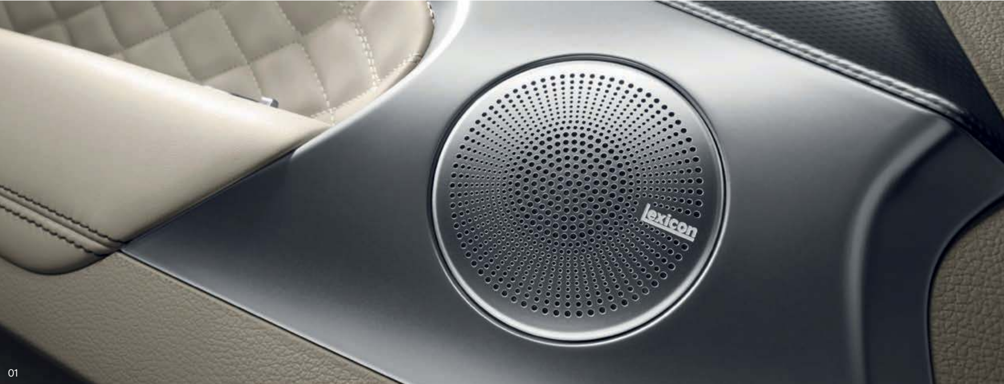
01. 15 Lexicon speakers system (Quantum Logic Surround) _ 15 Lexicon speakers with the latest Quantum Logic surround sound technology are positioned optimally for the best acoustic performance. Real stainless steel midrange speaker grilles reproduce a clear voice range that is close to the original sound. Subwoofers installed on the bottom of the driver's seat and front seat provide the deepest and richest bass sound experience.
