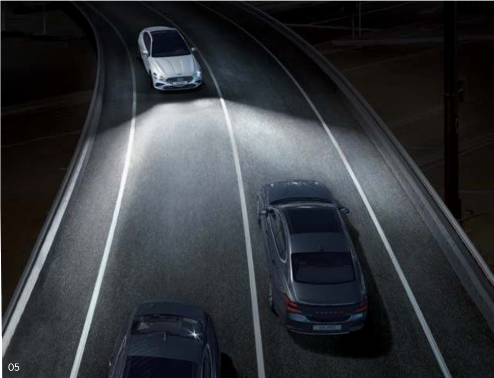
05. Intelligent Front-Lighting System (IFS) _ This system automatically activates or deactivates part of the high beam lights when it detects an oncoming vehicle or a vehicle ahead, to prevent glare for drivers of other vehicles. This supports safer driving at night as the high beam lights don't have to be adjusted manually.
