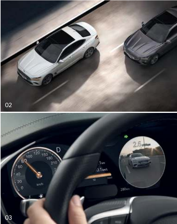
03. Blind-Spot View Monitor (BVM) system _ When the turn signals are activated to change lanes, video images on the center cluster show larger areas of the respective side/rear of the vehicle than the side-view mirrors to assist safe driving.
