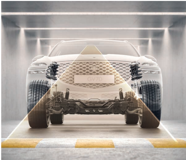
ELECTRONICALLY CONTROLLED SUSPENSION WITH ROAD PREVIEW
