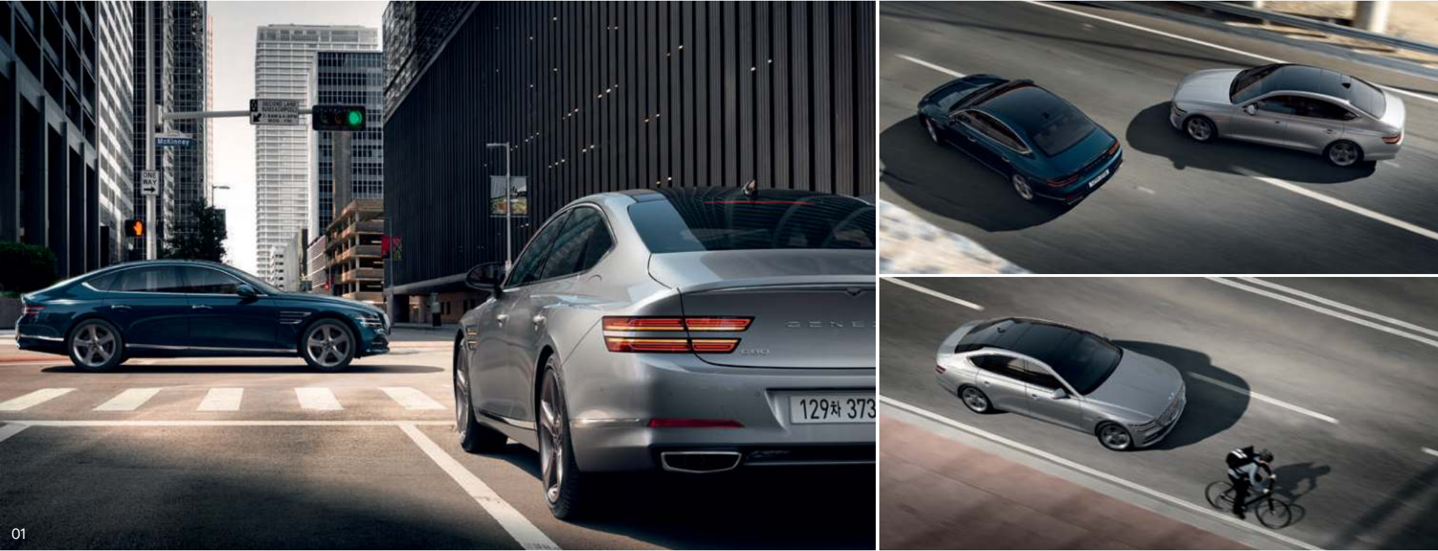
01. Forward Collision-Avoidance Assist (FCA) system (junction crossing, change oncoming, change side, evasive steering assist) _ This system helps to automatically bring the vehicle to a stop when there is a collision risk with another vehicle, cyclist or pedestrian that suddenly appears or stops ahead, or with vehicles approaching from the left or right side of an intersection. FCA helps to automatically steer the vehicle away from an oncoming vehicle or from a vehicle ahead in the adjacent lane if a collision risk increases while changing lanes, or when a pedestrian and/or cyclist gains proximity to a moving GENESIS G80 in the same lane.
