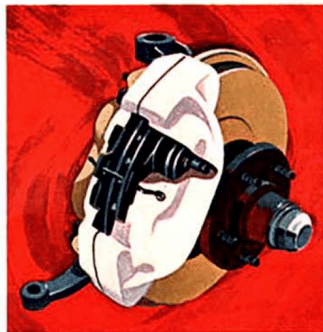
Front-Wheel Caliper-Type Disc Brakes for tough service.
