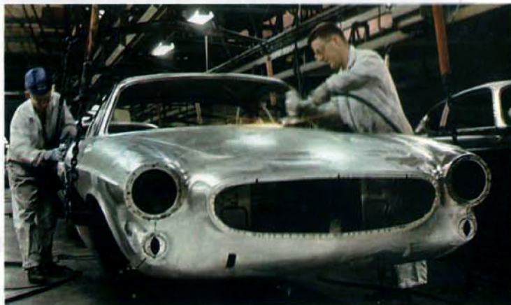
Integral construction body — one rigid unit for outstanding road-holding and excellent safety.
