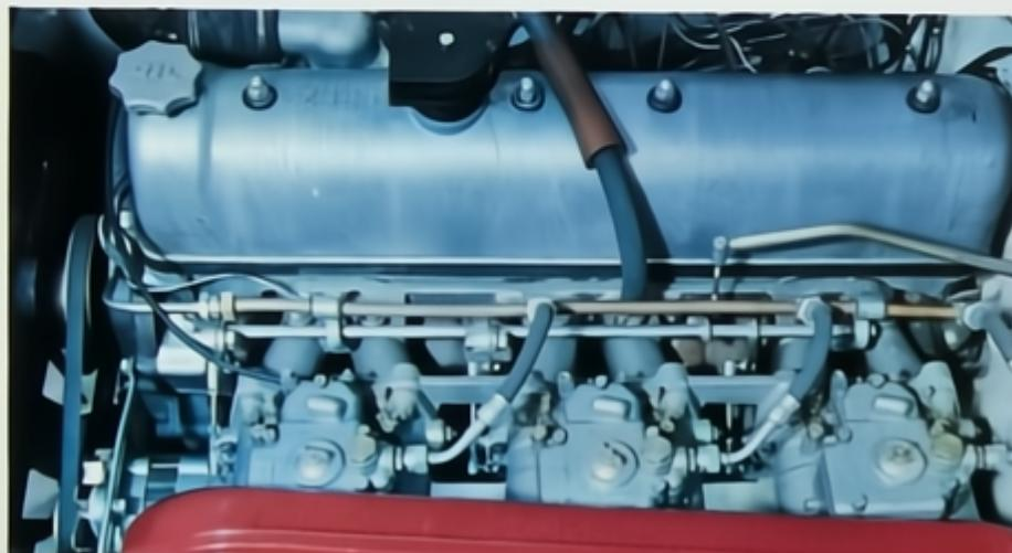
Three Weber side draft type carburetors are attached to the highly reputed model G7 engine to raise the compression ratio to 9.3:1. This OHC type, 6-cylinder, 2,000 cc, 127 HP engine gives a top speed of 180 km/h (111.5 mph), a max. climbing gradient of 50.2% and a max. torque of 17 m·kg (123 ft-lbs) at 4,400 rpm.
