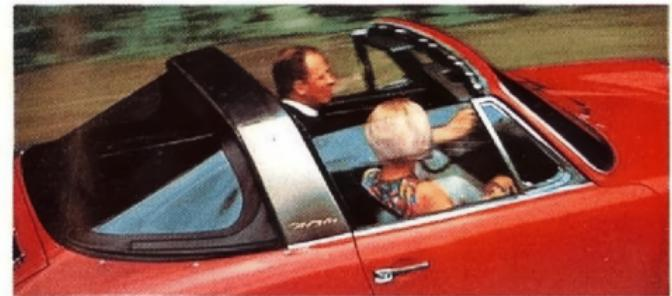
First of any convertible to have a roll bar built-in as an integral part of its design is the Targa, Porsche's four-in-one convertible. The bar, under a stainless steel, streamlined band, adds strength and safety to the rigid, unitized Porsche body while enhancing its lines.
