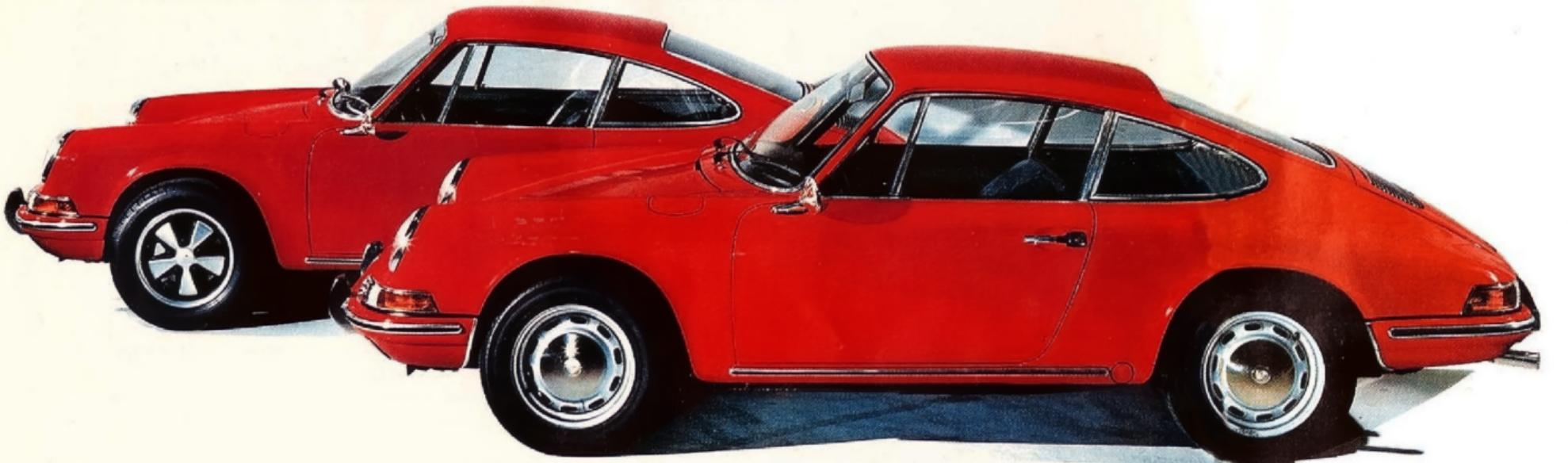
In appearance, the Porsche is still the Porsche. No one can mistake it. The newest versions sport slightly flaring fender skirts to accommodate the wider tires mounted on the new, wider wheels. Wider tires transmit the increased power of the latest 900's to the road and provide more friction surface for better braking.
