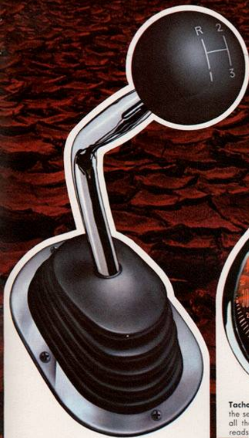
Three-on-the-floor makes it. New for '70. A three-speed fully synchronized manual transmission. Standard on the column with the 318 V-8. Optional on the floor with any Duster engine. (Standard on Duster 340.)
