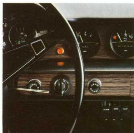
One more speed. Electric overdrive lets the 1800E go faster while the engine goes slower. Just flick the lever.
