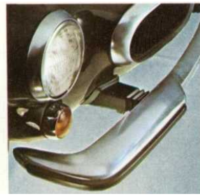
As to new bumpers aren't designed to bump but rather, to take a bumping. They're mounted on oil-filled, hydraulic shock absorbers and designed to take impacts at 5 mph (front) and 2.5 mph (rear).
