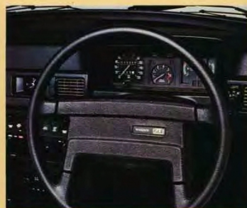
The centre of the steering wheel consists of a large pad which can absorb and spread the pressure exerted by a body if thrown forward.
