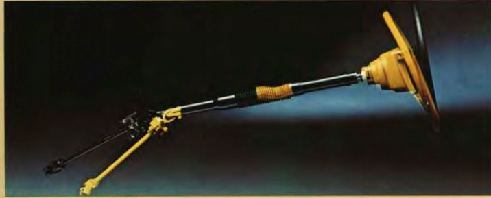
The steering wheel and steering shaft are designed to provide maximum safety in the event of a collision: The lower steering shaft section 'gives' way, the steering column slides forwards and downwards, the steering wheel attachment 'gives' so that the padded surface in the centre of the steering wheel has as large a contact area as possible.
