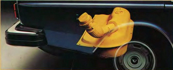
The fuel tank is placed close to the rear axle. It is completely separate from the passenger and luggage compartments.
