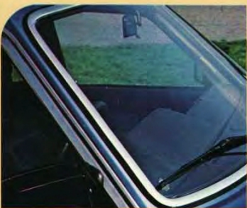
The windscreen is of high-impact laminated glass. The glass remains completely transparent even if it is struck hard by flying stones.
