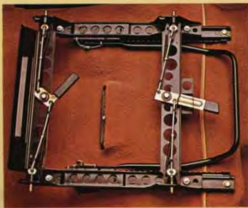
The front seat attachment is designed to withstand extremely high stress, such as the kind that occurs in accidents, without the seat loosening.
