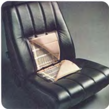
GLE MODELS HAVE A HEATED DRIVER'S SEAT TO WARM YOU IN THE WINTER. THE BERTONE COUPE HAS IN ADDITION A HEATED FRONT PASSENGER SEAT.
