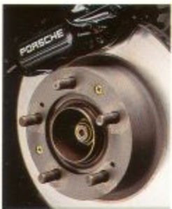
Front disc brake technology common to all 911s: four-piston fixed caliper, internally vented.
