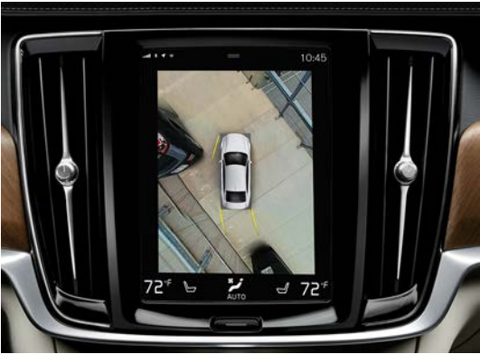
360° SurroundView Camera The 360° SurroundView Camera uses images from discreetly mounted cameras to create a bird's-eye view of your car and its closest surroundings. In the center display, you can see obstacles all around you, which makes it easier to park and maneuver in tight spaces.
