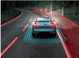
Run-Off Road Mitigation Stay safely on the road with this Volvo Cars safety innovation. If Run-Off Road Mitigation detects that you're about to leave the road unintentionally, it uses steering input and, if necessary, brake support to guide you back on track.
