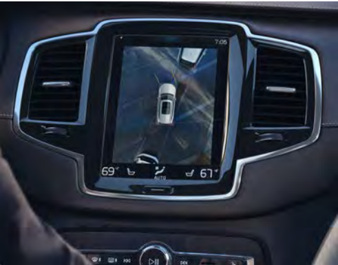
360° camera The 360° camera uses images from discreetly mounted cameras to create a bird's-eye view of your car and its closest surroundings. In the center display, you can see obstacles all around you, which makes it easier to park and maneuver in tight spaces.
