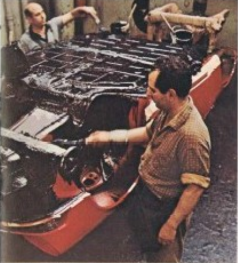
If the undercoating, 35 lbs. of it, hasn't been brushed on before the bell rings, one of the men will move on to the next station, along with the car, until it is.
