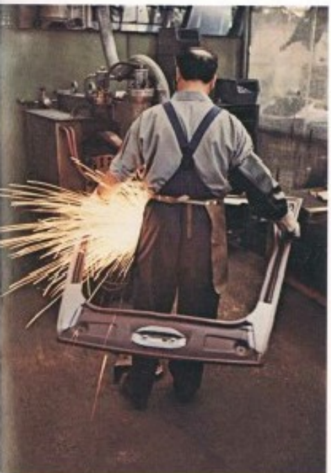
The Porsche hood frame is as rigid as the rest of the body, because it too is welded, not bolted.
