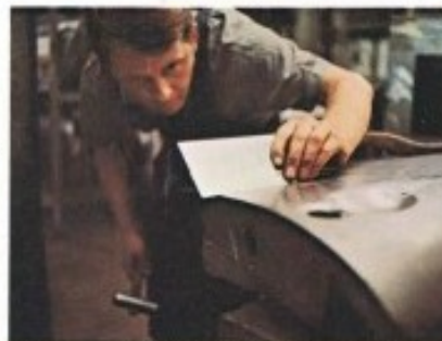
The door isn't finished until this man says so. And he says so when no light shows between the door and the template.
