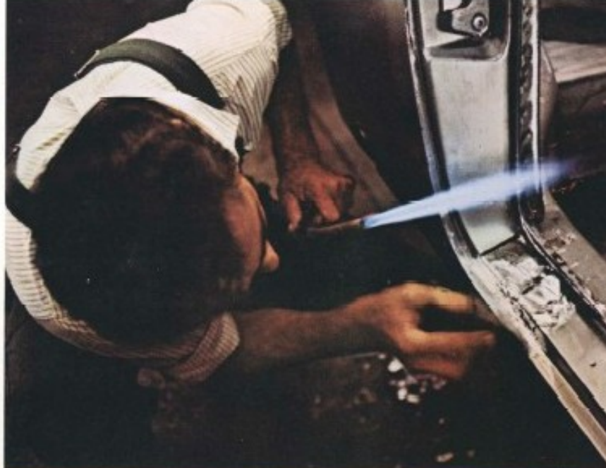
To make sure there aren't any spaces where there shouldn't be any spaces, this man fills them in with body lead or soldering tin.
