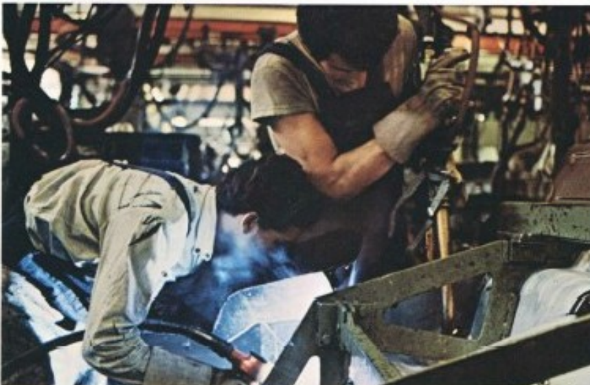
Why even old Porsche bodies don't rattle. A Porsche body being welded, not bolted.
