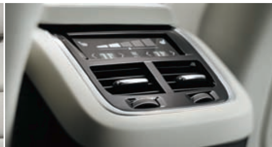
Thanks to the four-zone climate system, passengers in the outer two rear seats can set the temperature and fan speed to their individual taste – and the same goes for the driver and the front passenger.
