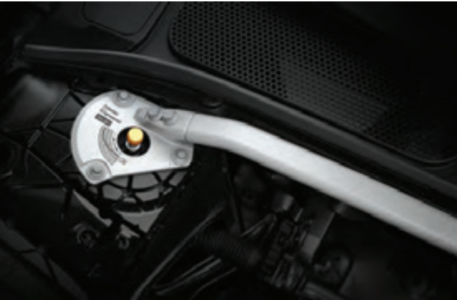
The front suspension is further stabilized by a Polestar Engineered strut bar. This contributes to even more precise, responsive steering characteristics at all speeds and more controlled handling through the curves.
