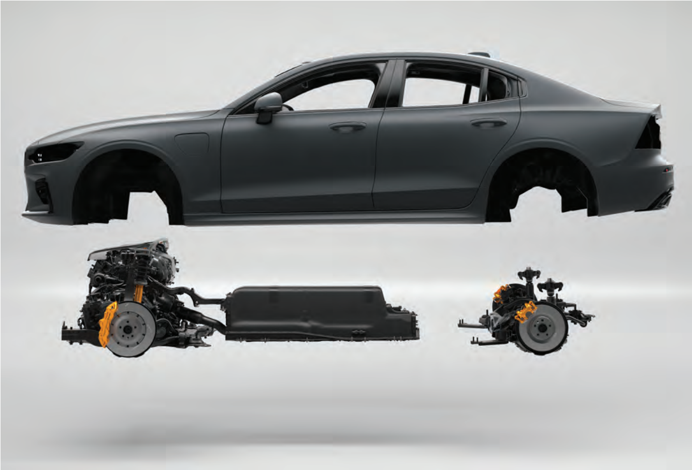
We created the Polestar Engineered Öhlins Chassis to give you the perfect balance of agility, control and comfort. The advanced Öhlins shock absorbers work together with the Polestar Engineered front and rear springs that stiffen up the chassis and lower the ride height. This gives a somewhat firmer and more composed ride with less roll and more grip when cornering. And for stable and predictable handling, the technical layout of the T8 Twin Engine AWD powertrain adds to even weight distribution and a low centre of gravity.
