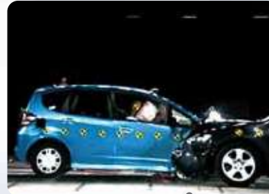
The Jazz goes through the most stringent tests at the Honda crash test facility
