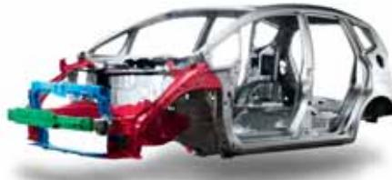
**ACE™ Body Structure.** The Fit's Advanced Compatibility Engineering (ACE) body structure disperses frontal impact energy to increase occupant protection and allow for collision compatibility between vehicles of different weights and sizes.
