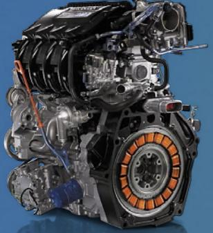
Integrated Motor Assist (IMA) is our proprietary hybrid system that delivers both exceptional fuel economy and extremely low emissions. The 1.3 litre i-VTEC engine serves as the main power source, providing the torque and acceleration you might expect from a 1.5 litre engine. But the Insight also has an electric motor that can run the car alone when you're cruising at low speeds and also provide additional power.
