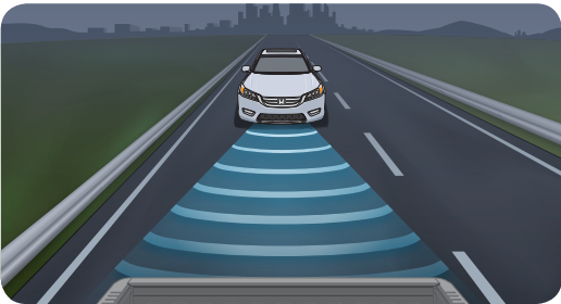
ADAPTIVE CRUISE CONTROL (ACC) 11 ACC electronically regulates your following distance in Adaptive Cruise Control mode, accelerating or decelerating depending on how close you are to the vehicle detected in front of you. (Touring)
