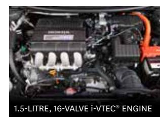
1.5-LITRE, 16-VALVE i-VTEC® ENGINE
