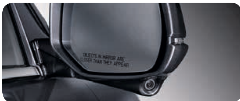
Honda LANEWATCH® A camera under the passenger-side mirror captures more of what's beside and behind you. It displays on your i-MID, revealing more than your mirror can. (EX and above)
