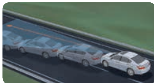
LANE DEPARTURE WARNING (LDW)⁹ A small camera searches for lane markings on the road. If it detects the driver making an unindicated lane departure, visual and audible alerts will signify the departure. (EX-L and above)
